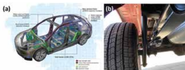
Figure 13. (a) The 2022 BMW iX battery-electric sports activity vehicle (SAV) features a multi-material combination of metals and composites in its innovative Carbon Cage. (b) Rassini's 1+C hybrid leaf spring features a single steel parabolic main plate and a flat glass fiber composite helper plate to provide suspension on the rear wheels of the Ford F-150 pickup truck
