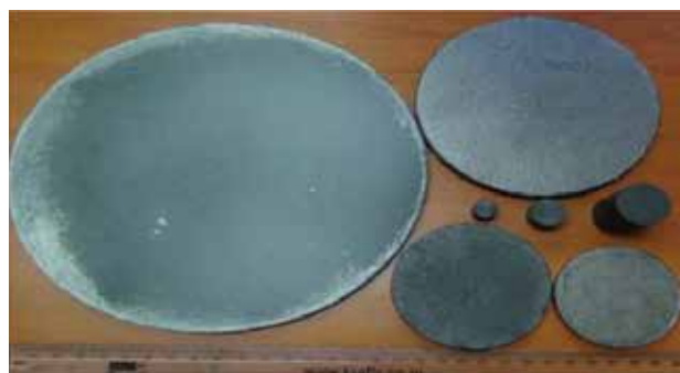
TiB 2 dense shapes of different sizes
