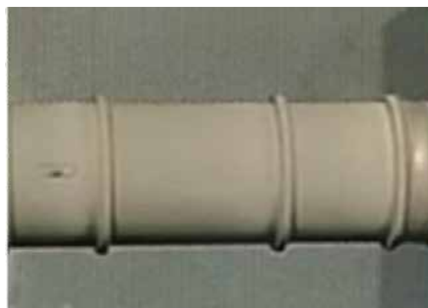
Detonation spray coated pump shaft of nuclear power plant
